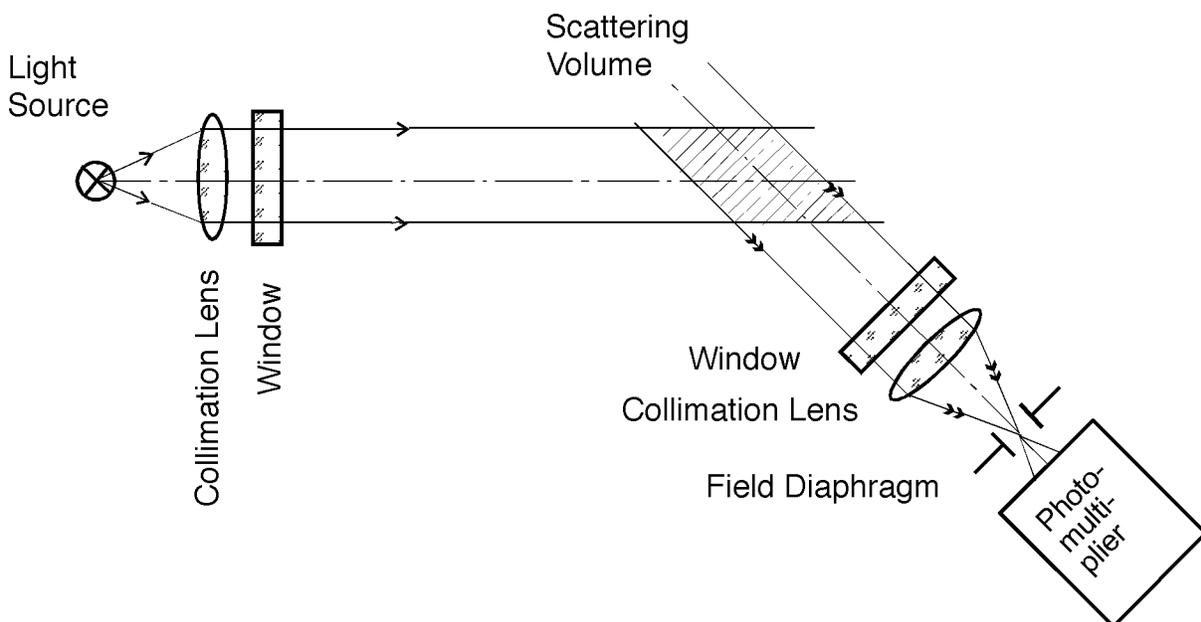
Fig. 1. Old schematic for volume scattering function measurements
