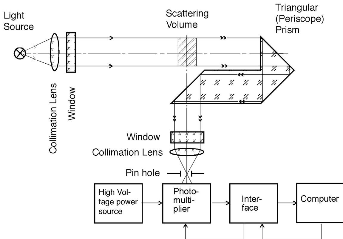
Fig. 2. Proposed schematic for volume scattering function measurements.
